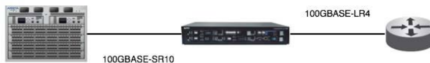
Figure 2: LD 400L converting SR10 to LR4 for interconnecting to other devices as required.
