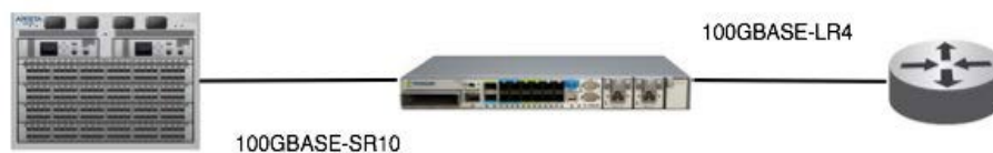
Figure 2: Pair of PL-1000GMs providing distance extension via an LR10 between Arista 7500E's
